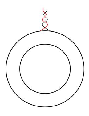
55mm LINE CT INNER DIA.-55mm DUTER DIA.-85mm
