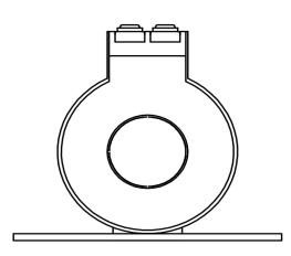
20mm LINE CT INNER DIA.-20mm DUTER DIA.-47mm
