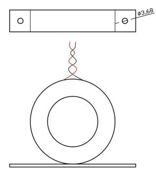
35mm LINE CT INNER DIA.-35mm DUTER DIA.-59mm
