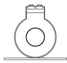
20mm LINE CT INNER DIA.-20mm DUTER DIA.-47mm
