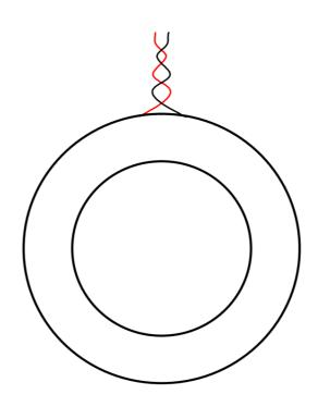
55mm LINE CT INNER DIA.-55mm DUTER DIA.-85mm
