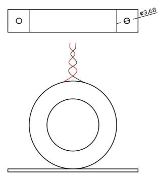
35mm LINE CT INNER DIA.-35mm DUTER DIA.-59mm
